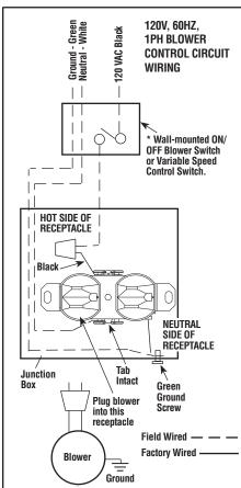
\*An ON/OFF Wall Switch is used with the FBK-100 kit (field provided or sold separately - order P/N 85L87); A Variable Speed Control (provided) is used with the FBK-200 kit. The installation of these kits also require a Junction Box / Electrical Kit, not included. See *Page 15* for ordering information.
